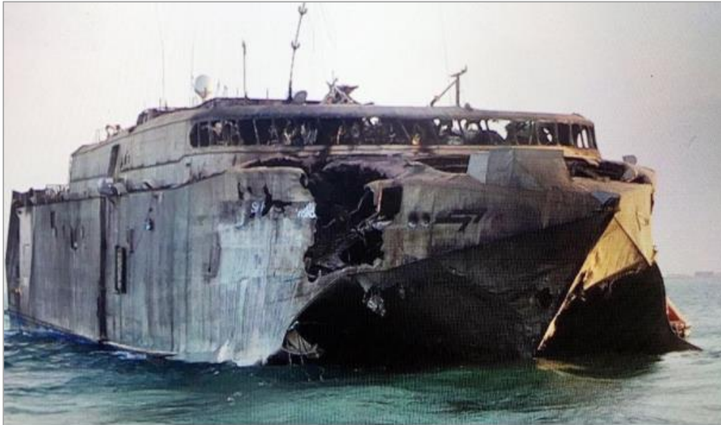
Image showing the impact damage of the missile on HSV -2's Starboard bow
