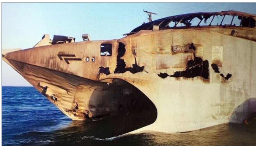
Image showing the exit blast damage on HSV -2's Port bow
